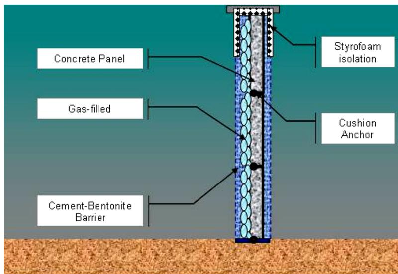
Figure 16. Gas cushion system with flexible cushions attached to stiff, prefabricated concrete panel.
