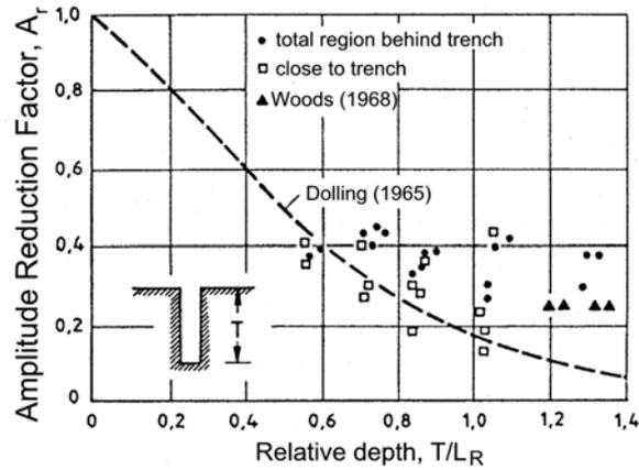
Figure 4. Results of vibration isolation model tests with open trench (Haupt, 1981). Results from tests by Woods (1968) and reduction curve suggested by Dolling (1965).
