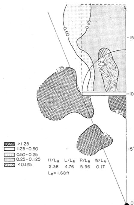
Figure 2. Passive isolation test: vibration amplitude reduction contours, (from Woods, 1968). H = trench depth, LR = length of Rayleigh wave, L = trench length, i = trench width.
