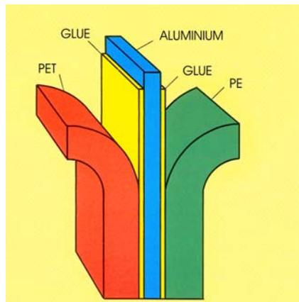
Figure 15. Laminate membrane used for gas cushions. Components: PTE (Polyester, Oriented, Primed + Polyethylene), Glue layer, Aluminium foil, Glue layer; PE (Polyethylene, Low Density Polyethylene).
