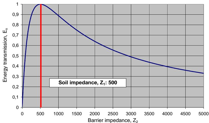
Figure 6. Energy transmission in soil with impedance  $Z_1$ , across a barrier with variable impedance  $Z_2$ , cf. Eq. 5.
