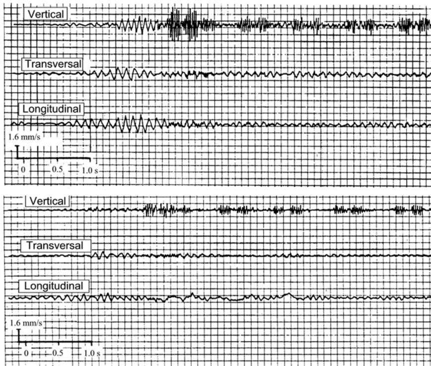
Figure 9. Vibration velocity record before and after installation of gas cushion screen on first building floor.
