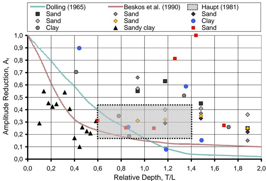
Figure 14. Isolation effect of gas-filled cushions in different soils and vibration sources. The variation of data points is caused by the fluctuation of the frequency spectra, from which the amplitude reduction factors were determined.
