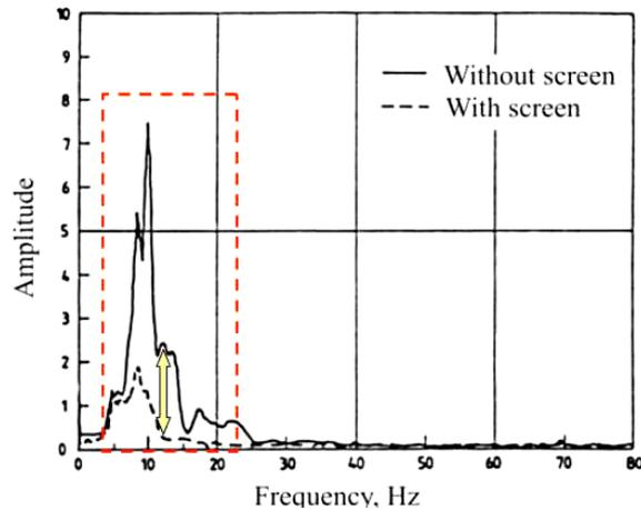
Figure 5. Determination of vibration isolation effect from the frequency spectrum of vibration signal. The dashed zone indicates the frequency range of interest.
