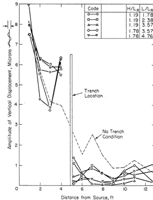
Figure 3. Amplitude of vertical vibration amplitude vs. distance from the source for five tests, (from Woods, 1968).
