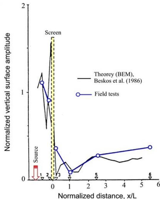
Figure 11. Results from vibration isolation tests in Uppsala, Sweden. The test results are compared with theoretical predictions using a 2D BEM analysis, Massarsch (1986).
