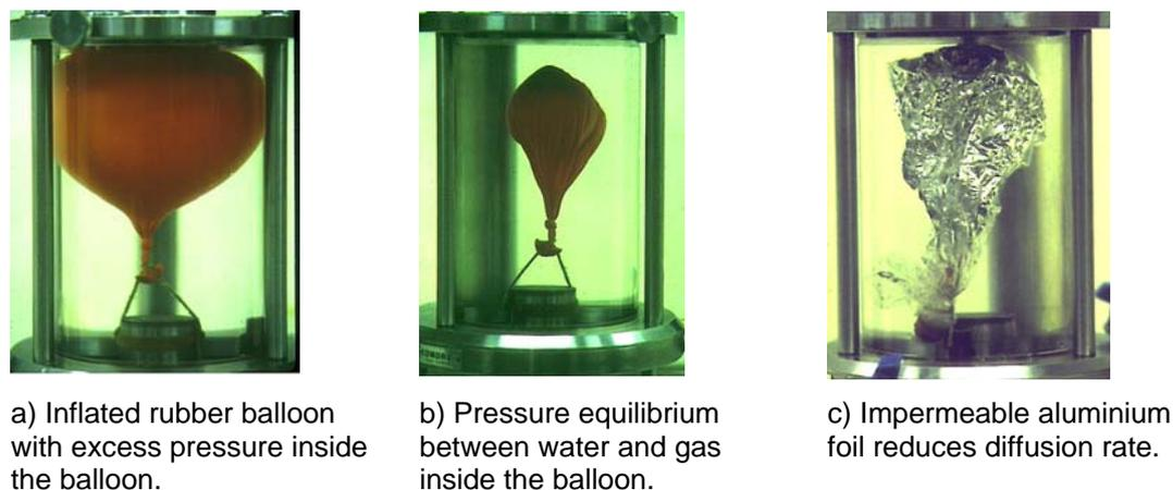
Figure 7. Illustration of gas cushion principle.
